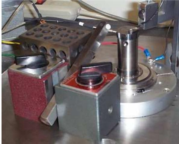
**Figure 10: Dynamic Stiffness Test Setup**
