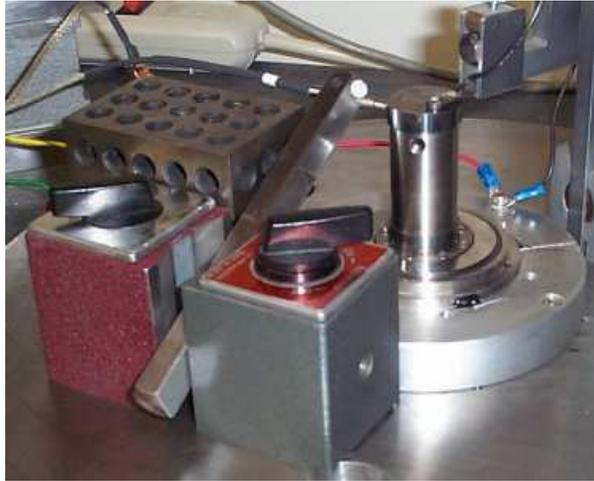
**Figure 10: Dynamic Stiffness Test Setup**
